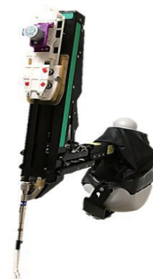
Fig. 1: The CTSM based Flexible Manipulator on the PSM
